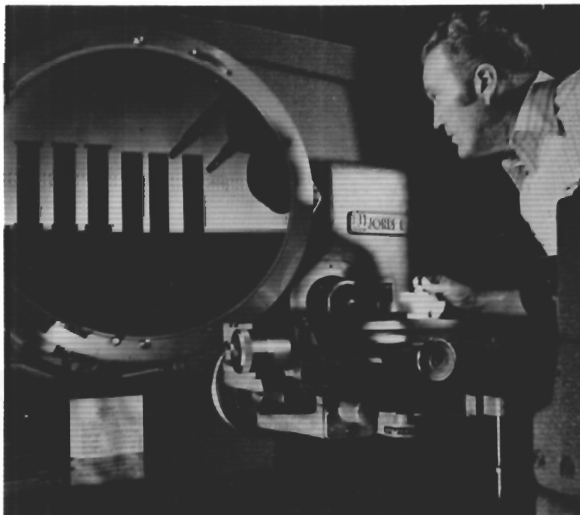
To insure long-lasting computer tapes and trouble-free reels, critical components are inspected with an optical comparator.
