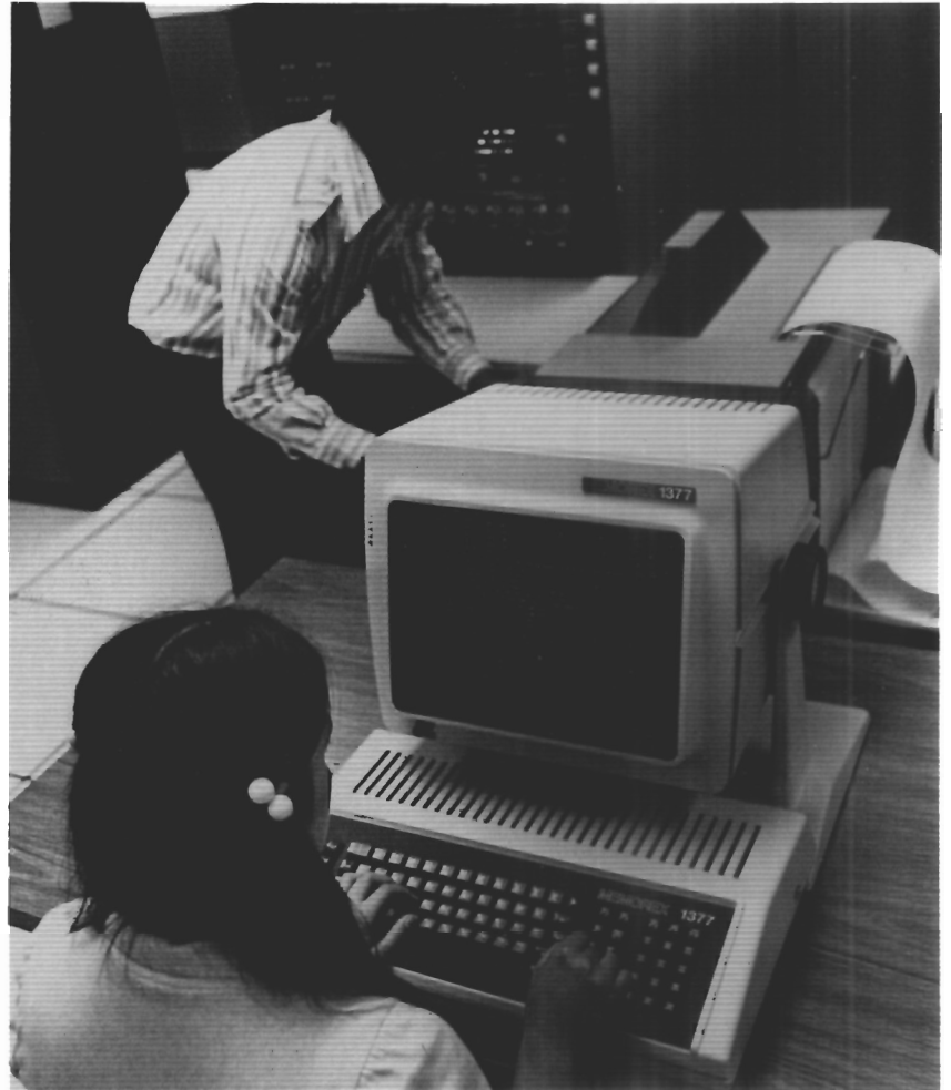
The new 1377 Display Station offers exclusive features including a tiltable screen for operator convenience.
