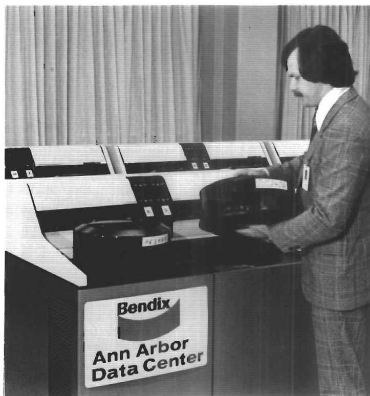
One of the 367X series of proven, highly reliable Memorex disc files, the 200-megabyte 3675 model is in operation at Bendix Corporation, among the many customers for this storage subsystem.
