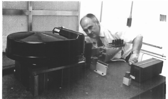
Precise alignment of heads in the 3650 Head Disc Assembly is accomplished by this servo-writer which uses a laser beam positioning device.
