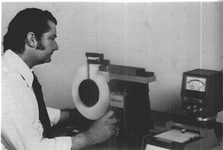
For superior operation, the dimensions of the new Super Reel are inspected by special electronic gauges. The diameter of the reel hub is checked to an accuracy of .00015 of an inch.
