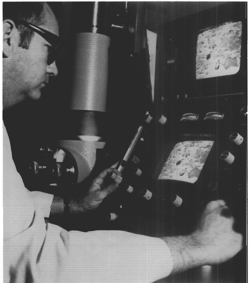
Essential tool in quality analysis for computer tape is the new scanning electron microscope.
